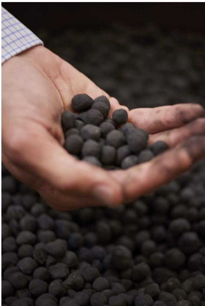
Iron pellets that fill the battery are abundant and inexpensive and could hold electricity for days or weeks.
