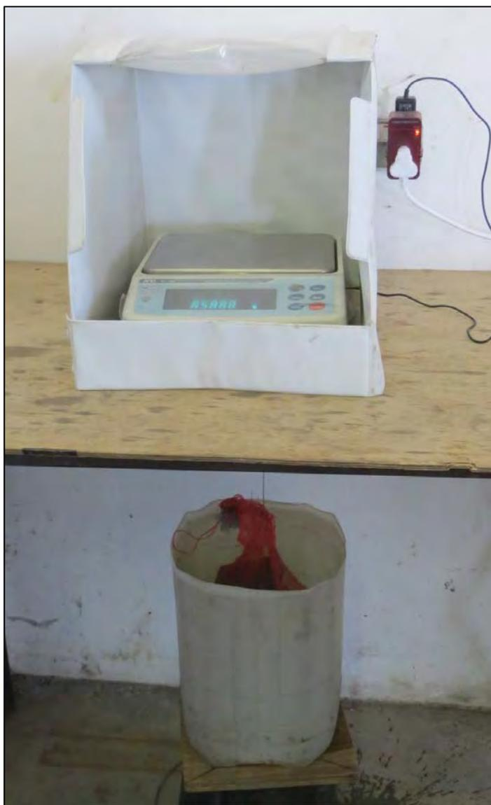
Figure 10-3: Density measurement equipment (Source: Gcwihaba protocols, 2014)
