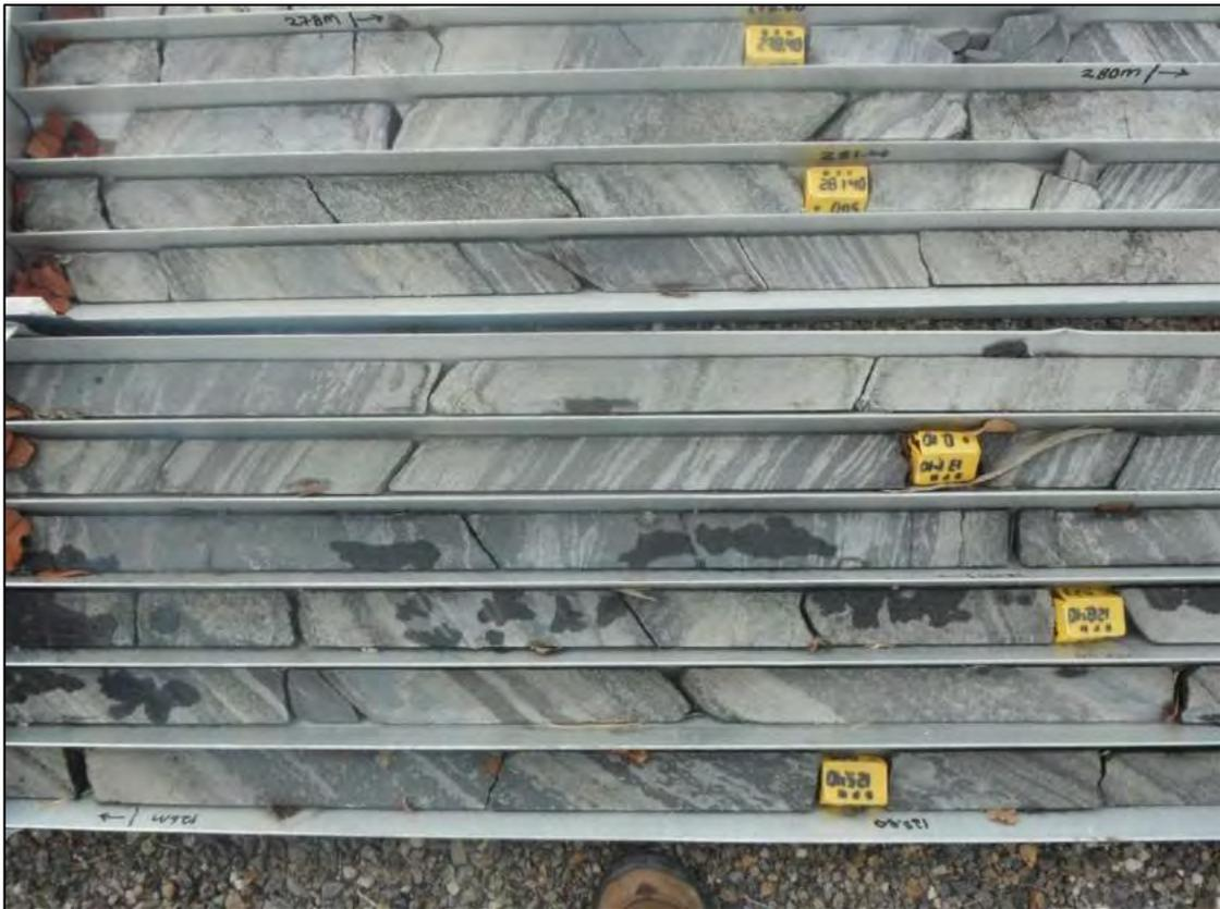
Figure 6-10: Banded magnetite - geodomain MBA (Source: SRK site visit, 2014).
