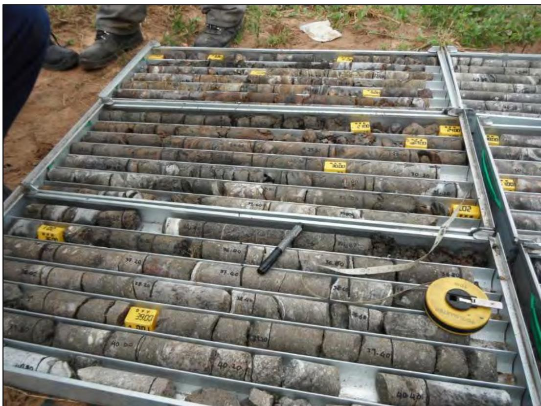
Figure 9-2: Example of drill core and core boxes (Source: SRK site visit, 2014).
