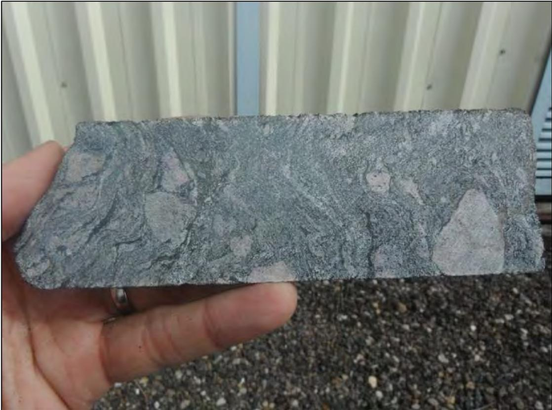
Figure 6-12: Diamictite Magnetite Schist - geodomain DIM (Source: SRK site visit, 2014).
