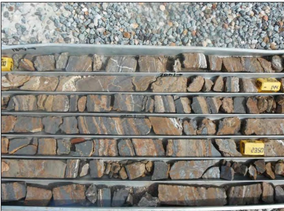
Figure 6-11: Weathered Banded magnetite - geodomain MBW (Source: SRK site visit, 2014).
