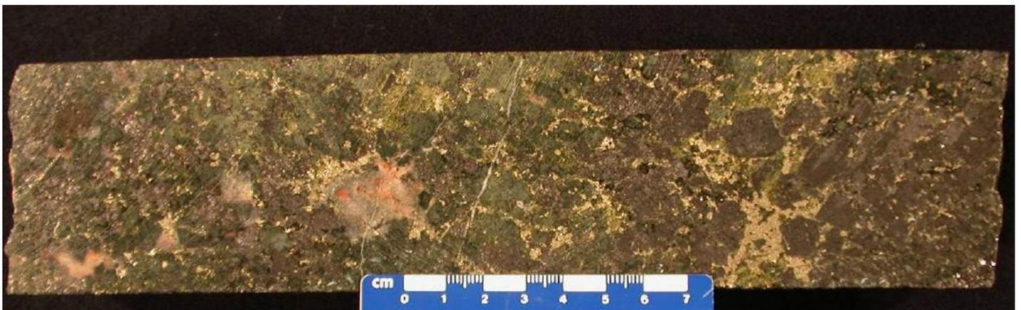
Figure 11.3 Disseminated sulphides in coarse meta-gabbro.
