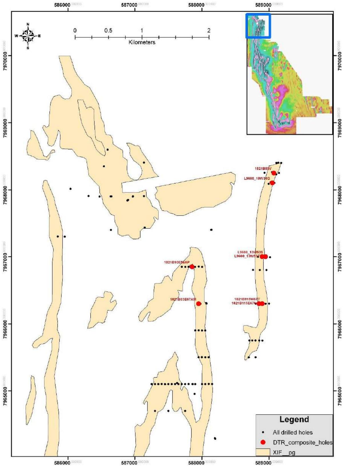
**Figure 1: Ground magnetic interpreted first vertical derivative outline, indicating where the XIF magnetite mineralisation body is interpreted below the Kalahari cover. Black dots represent all holes drilled in the area and the red dots are DTR composite holes.**
