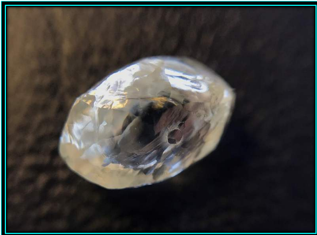
IMAGE 7: A CIRCULAR IMPACT NOTED ON A DODEC IN THE HISTORICAL SAMPLE
